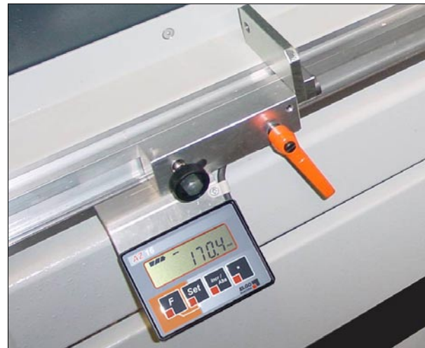
AZ16E application example: manual gauge
