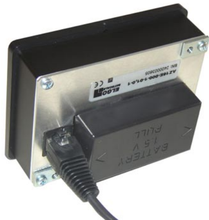
AZ16E rear: with battery case and plug connector
